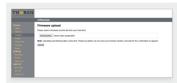
If a new firmware is available for your device you can flash it using the web interface. Go to the Menu Firmware and select the file you want to flash. Click the Upload button and wait until a confirmation appears that the upload was successful.
