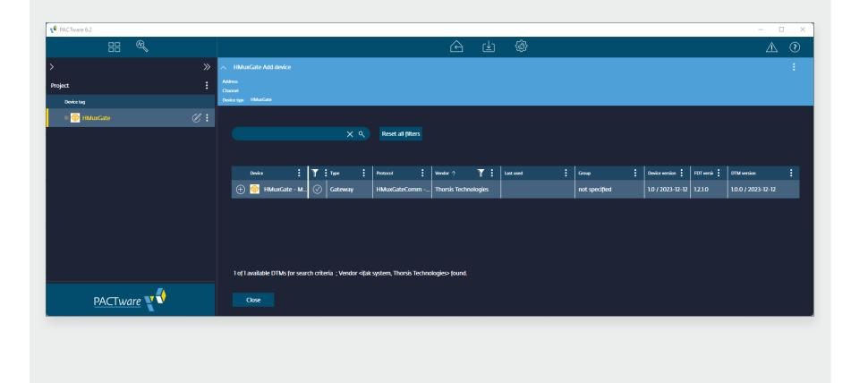
Before you can go online with the new device, you still need to enter the IP address of the isHMuxGate. In order to do so, select the Parameter menu item from the context menu.
