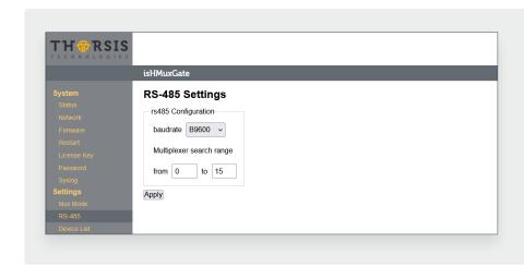
On this page the user can set the baud rate on the RS485 connection to the HART multiplexers. Furthermore the user can select the address range of the HART multiplexers.
