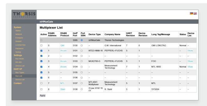
On this page the isHMuxGate shows all HART multiplexers connected to this gateway. The number of multiplexers shown here depends on the "Multiplexer search range" in the RS485 settings (see chapter 3.7 "RS485 Settings" on page 17).
