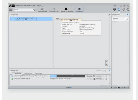
The active HMuxGates and HART multiplexers are found and listed. The connected HART devices are displayed under the modules.
