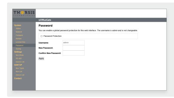
To enable a global password protection for the isHMuxGate web interface, click on the Password menu on the left. Activate the Password protection by clicking in the checkbox. Enter your password and repeat it in the field below.
