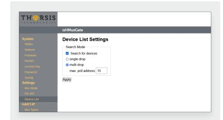
The isHMuxGate keeps track of all HART instruments wired to the connected HART multiplexers.
