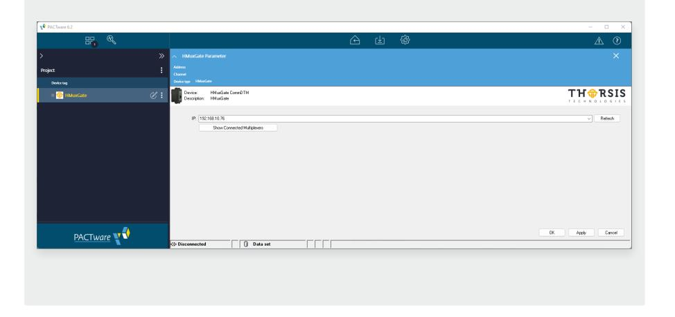
For informational purposes you can press the button (Show Connected Multiplexers). This will present a list of all HART multiplexers currently connected to the selected isHMuxGate. PACTware 6.2 == TH TRSIS HMuxGate CommDTM Description: HMuxGate IP: 192.168.10.76 Refresh 5100 - 5700 5101 - KFD2-HMM-16 5103 - MUX2700-G 5104 - MTL4850 Multiplexer 5108 - IS pac 9192 16 ch Hide PACTware 🛂 OK Apply Cancel Disconnected Data set
