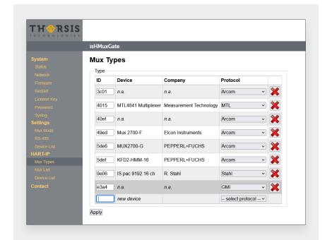
The isHMuxGate contains a list with known HART multiplexers. If necessary additional HART multiplexers can be added to this list. In order to do so, the user needs to enter the Expanded Device Type ID and select the protocol which the multiplexer is using on RS485 for communication.
