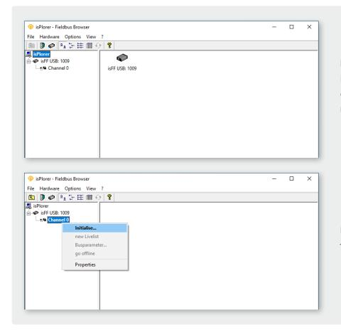
Before starting the software, you should connect the isFF USB Interface to your PC. After the subsequent start of isPlorer the device appears on the left in a tree view along with the FF-connector accompanying the appliance.
