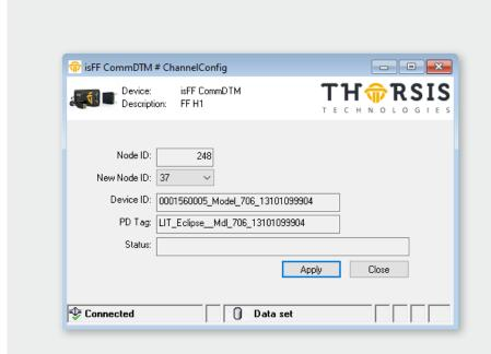
With the help of this ActiveX the Node ID for an FF device can be set to a new value. This menu is only available for slaves without Device DTM.
