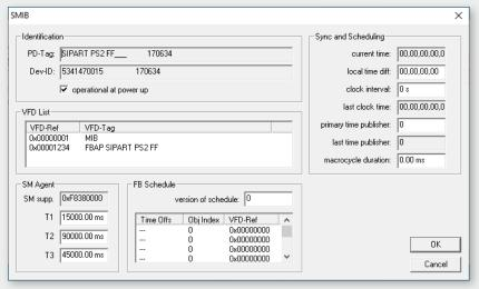
In this view, it is possible to change the address and PD-Tag of a field device and to display system information of the field device.
