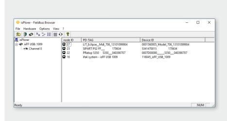
After completion of the initialization phase, the program is Plorer scans the bus for connected field devices and displays them in the right pane. In the detail view, further information such as the device ID or the PD-Tag of the connected field devices are shown.
