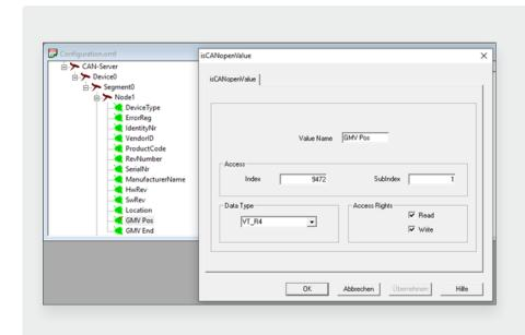
For definition of CANopen parameters, the user configures the index and the subindex as well as the datatype. For configuration of PDOs or basic CAN messages the user needs to configure the CAN message identifier instead of the index and subindex.
