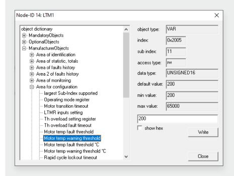
The user can also configure all communication parameters such as COB-IDs, Node guarding, Heartbeat or define the PDO mapping.
