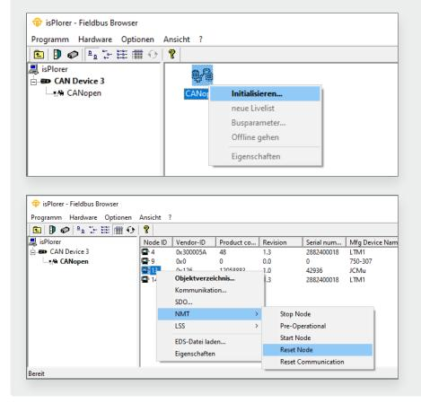
Before starting the software, you should connect the isCAN USB Interface to your PC. After starting isPlorer, the device appears on the left in a tree view together with the CAN connection associated with the device.
