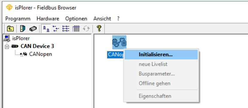
Before starting the software, you should connect the isCAN USB Interface to your PC. After starting isPlorer, the device appears on the left in a tree view together with the CAN connection associated with the device.
