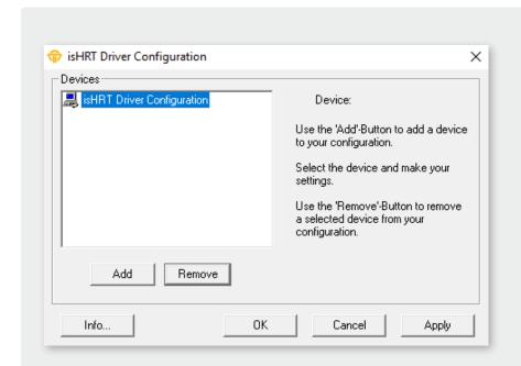
The configuration software isHRT Driver Configurator is provided in order to adapt the DLL access to your hardware. It is installed in the Start Menu. This dialog based application allows the easy addition and removal of HART interfaces. It also checks the available resources of the system.
