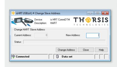
This ActiveX can be used to change the poll address of a HART interface. This Menu is only available for Slaves without Device DTM.
