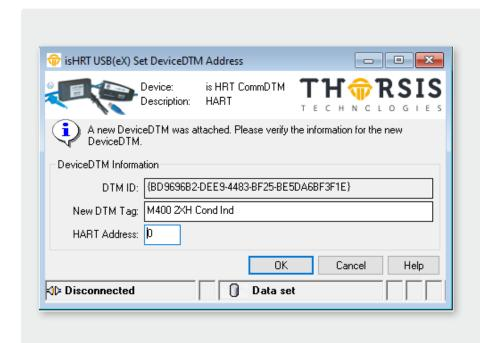
When a DeviceDTM is connected to the isHRT CommDTM then an ActiveX is opened, that allows to set the tag and the slave address of the DeviceDTM.
