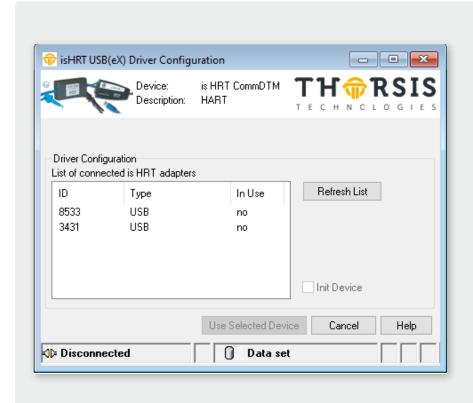
This dialog is used to select one of the connected HART communication interfaces of Thorsis.
