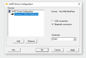
When selecting a Bluetooth connection, you must select the assigned COM port. You can also do this under Control Panel / Bluetooth / network access devices.
