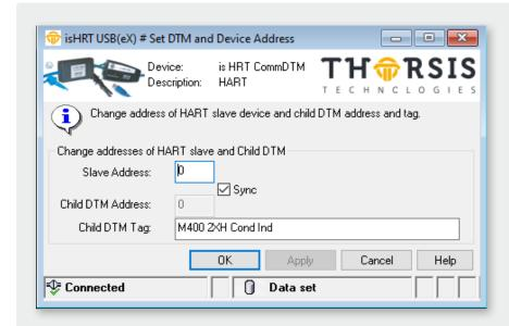
The new device address must not be in use and no DeviceDTM may have open connections to the source address. The isHRT CommDTM checks these requirements before the address change is attempted. If any of these requirements is not fulfilled or the change of address itself fails for other reasons, then an error message is displayed in the status field.
