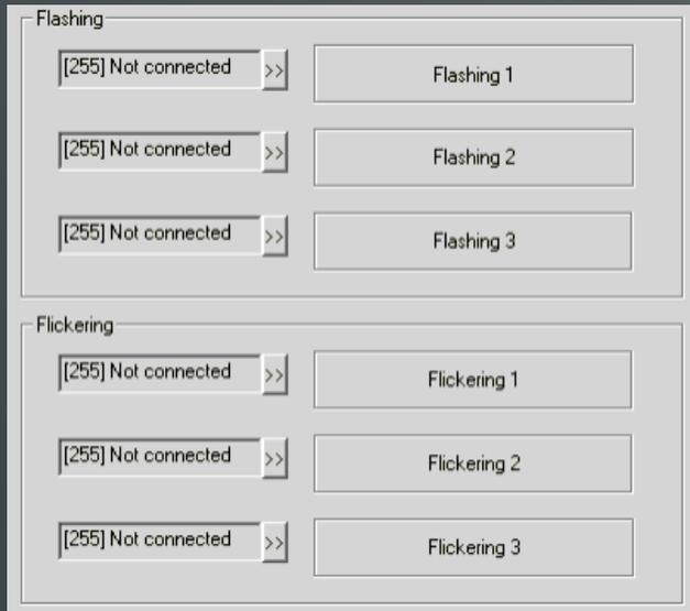
Flashing and Flickering are functions which you can assign, for example, to LEDs 1-3 of the operator panel or to the relay outputs. It is thus possible to indicate various different statuses. A total of 6 functions of this type are available. The flashing frequency is approx. 2Hz, and the flicker frequency approx. 8Hz.
