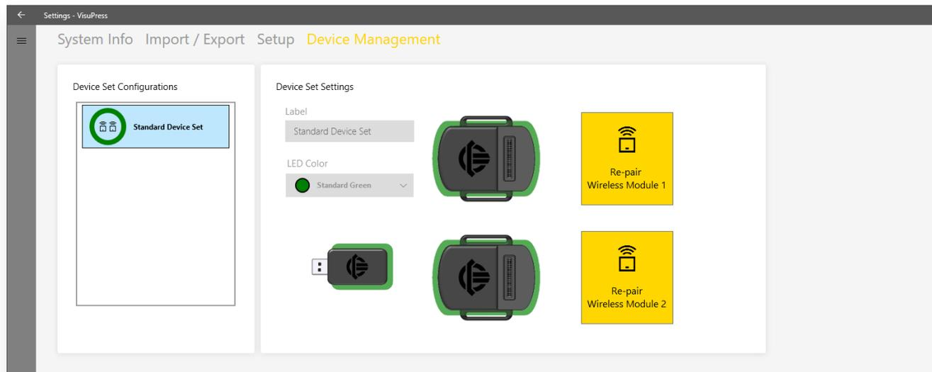
After successful pairing, the Master Module pulses, the Wireless Module and the associated symbols in the connection dialog in the LED color of the device set. Carry out the steps again to pair the other Wireless Module with the USB Master Module.
