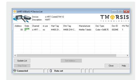
The isHRT CommDTM offers in addition to the function ScanRequest an own ActiveX to scan the HART bus for devices. This ActiveX provides information about HART devices (vendor, type, channel information) that are connected to the HART networks. If this ActiveX is called in an offline situation, it provides a list of Child-DTMs, all with no associated device.
