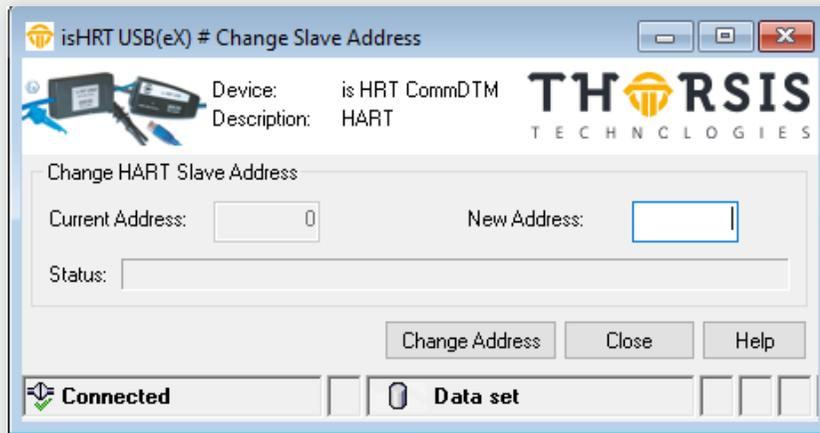
This ActiveX can be used to change the poll address of a HART interface. This Menu is only available for
