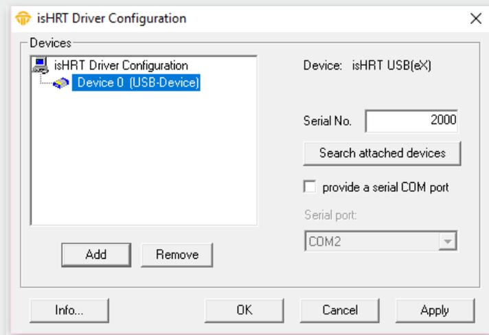
The device can work like a serial modem under the operating systems Windows 7, 8, 10 and 11. In order to facilitate this, it offers a serial COM-port so that already existing applications can be used without any changes. The serial COM-port can be selected. The configuration software checks the available COM-ports to avoid an address conflict.
