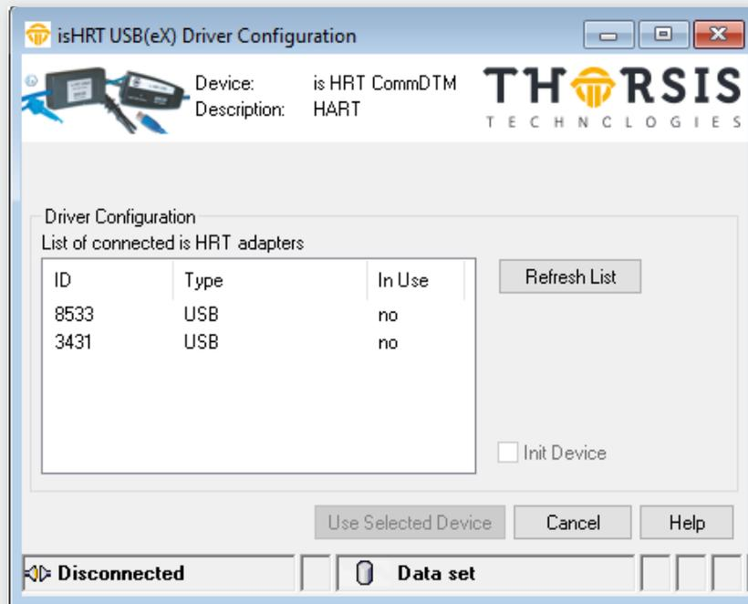
This dialog is used to select one of the connected HART communication interfaces of Thorsis.
