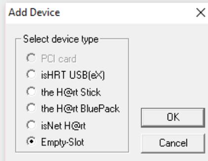
The empty device does not contain any resources. It serves as a substitute for device numbers not yet assigned. Using empty slots enables a free enumeration of devices by inserting empty devices between existing ones.
