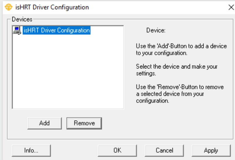
The configuration software isHRT Driver Configurator is provided in order to adapt the DLL access to your hardware. It is installed in the Start Menu. This dialog based application allows the easy addition and removal of HART interfaces. It also checks the available resources of the system.
