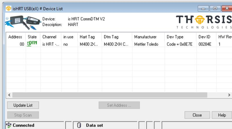
The isHRT CommDTM offers in addition to the function ScanRequest an own ActiveX to scan the HART bus for devices. This ActiveX provides information about HART devices (vendor, type, channel information) that are connected to the HART networks. If this ActiveX is called in an offline situation, it provides a list of Child-DTMs, all with no associated device.
