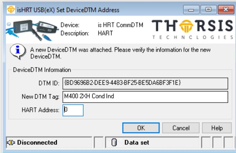
When a DeviceDTM is connected to the isHRT CommDTM then an ActiveX is opened, that allows to set the tag and the slave address of the DeviceDTM.
