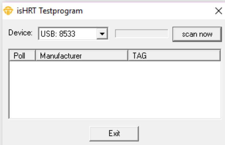
The correct installation and functionality of isHRT USB can be checked with the test application “isHRT Testprogram” in the driver software.
